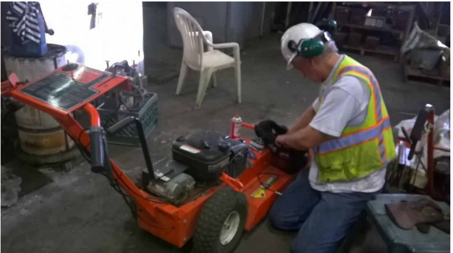
Steve replacing filters
